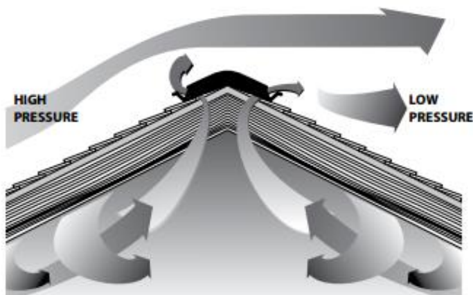
Figure 7-9: Wind passing over the externally baffled Ridge Vent creates low pressure at the vent's openings, which causes air to be "lifted" or pulled out.
